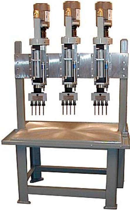
An AutoDrill designed Multiple Spindle Drilling Head system helped a customer fabricating doors to significantly increase their production drilling capabilities. The Multi-Drill fixture is capable of drilling all the hinge holes on a door in three separate hinge locations simultaneously. Multiple spindle drill heads and AutoDrill self-feeding drills reduce the multiple step operation to a single step.
